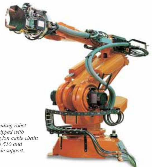
Circular nylon chains on welding robots.
