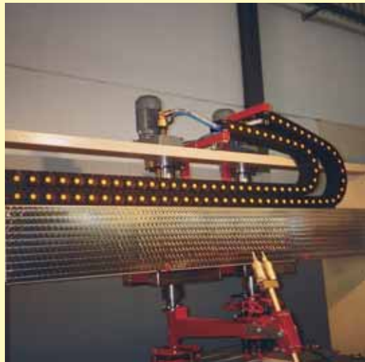
Model 700 chains in nylon superimposed on a machine which works with marble.
