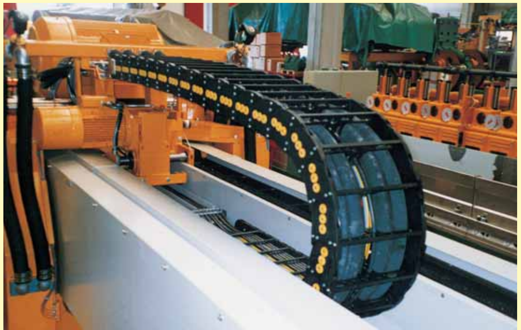
Nylon chain, type 310, in a self-supporting state.
