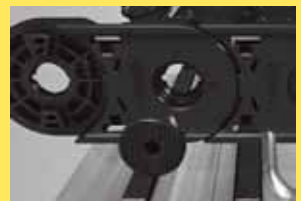
Easy opening of the pin junction.
